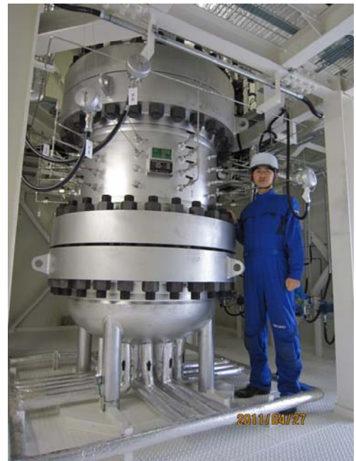
A large-scale experimental apparatus to simulate gas production processes from methane hydrate sandy sediment
